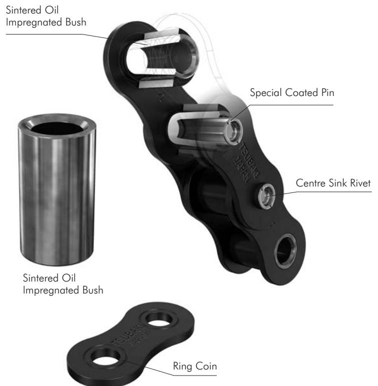
Fig. 10 Basic Construction
